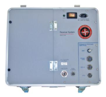
The MPSR is a durable surface receiver providing pulse detection, tool configuration, and logging-while-drilling capability.
